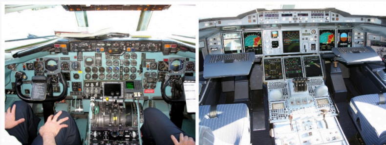
Figure 5.27 Airplane Cockpits. Initial design of the airplane cockpit (left); the digital design of the airplane cockpit (right), which has taken human factors into account.
